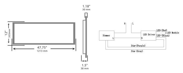
1x4 Field Tunable (watt and Color Temp.) Backlit LED Panel
