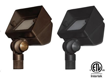
The Metropolitan wall wash comes with clear and frosted lenses. The lens is gasketed onto an angled shroud. Crafted from cast brass. A heavy-duty composite stake is included, and other mounting options are available. Tilt angle adjusts securely with a brass knob. Can be used for accenting building and barrier walls, as well as for lighting landscape features from below. A variety of LED bi-pin lamp intensities and hues are available.
