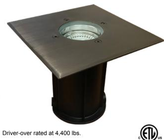
The Wentworth well light has an easily adjustable gimbal mechanism that allows precise aiming of the lamp for angled uplighting. Cast brass faceplate with a gasketed heavy-duty composite body. Can replace a standard 6-inch-square driveway paver.
