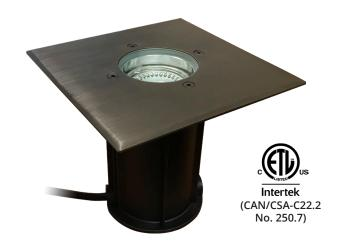
The Wentworth well light has an easily adjustable gimbal mechanism that allows precise aiming of the lamp for angled uplighting. Cast brass faceplate with a gasketed heavy-duty composite body. Can replace a standard 6-inch-square driveway paver.
