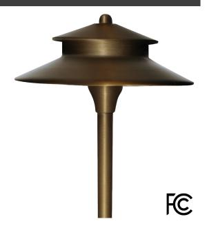
The Hemingway path light features an 8.5" diameter cast brass hat. Its underside is a powder-coated reflective white surface. 3W integrated LED with a 2700K or 3000K color temperature.
