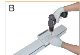
Following the template, secure the base plate onto the fixture
