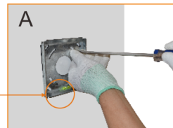
Uninstall the mounting bracket from fixture base plate by unscrewing the 2 hex socket studs.
